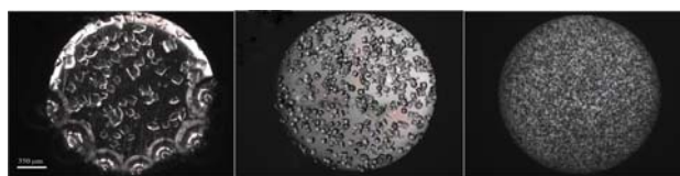
Fig. 1 Lysozyme crystals formed at an electrode surface after 2 h. From left to right: 5 \mu A applied current; no current; and no current with solution pH of 3.5. Scale bar shown is 350 \mu m.
